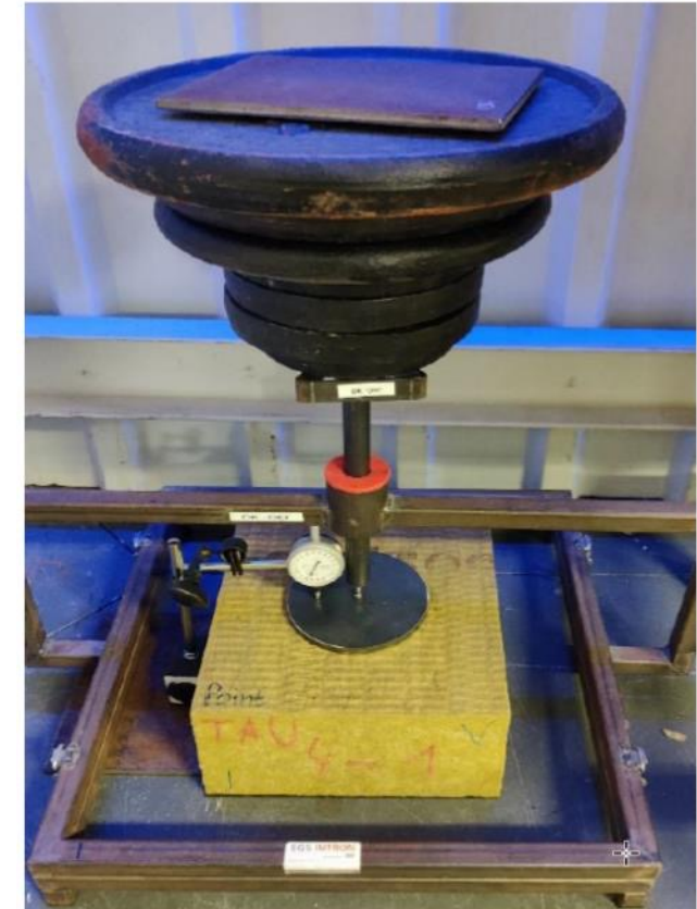
Figure 1: Test set up with a point load.
